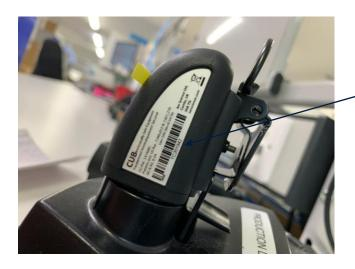
The Serial Number is located underneath the barcode. TC – 6 numbers (TC-XXXXXX)
