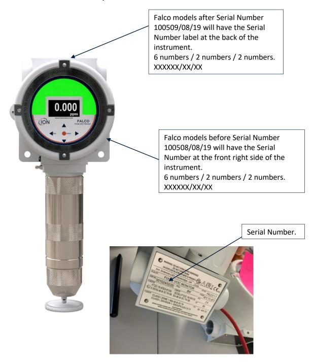
Whether this label is on the side or the back of the instrument, it will still look the same and the Serial Number is located in the same area on the label.
