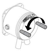
Turn counter-clockwise to unscrew the front cover.
