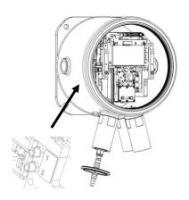
Ensure the pneumatic tubes are properly identified for later connection to the correct connectors.
