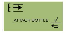
Attach the bottle before you start calibration. This ensures that benzene is flowing through the Titan 2 system before the start of the calibration.
